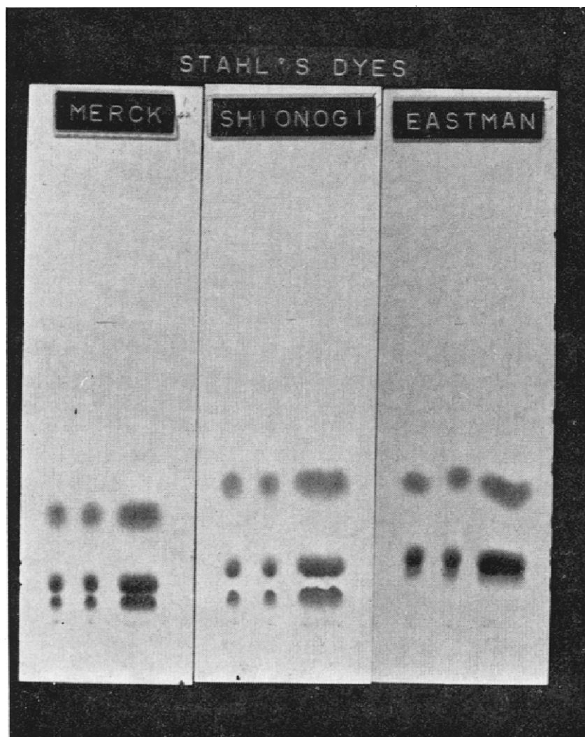
Fig. 1. Separation of Stahl's dyes on glass bases and polyester base. Left to right: Merck pre-coated glass plate, sintered plate, and Eastman chromagram sheet. Solvent: benzene. Dyes separated in order of decreasing R_f values: Butter Yellow, Sudan Red G and Indophenol.
